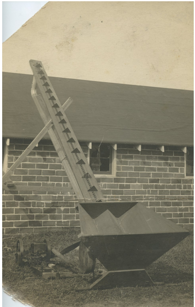
J.B. Majerus Portable Grain Elevator, which he invented and patented in 1919
